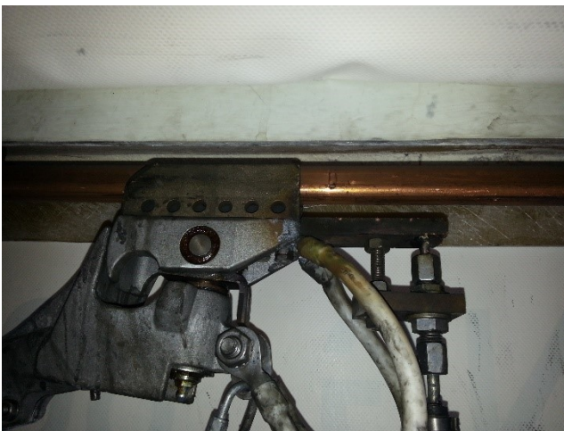
Pantograph converted to spray head
